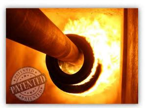
PRECALCINER KILN SYSTEMS The suspension burner is designed to burn whole tires in the calciner of the kiln. The burner includes a two gate airlock chamber, suspension fork assembly, automatic ram, weighing system, controls, and automatic fork cleaner. The burner is designed to mount to an AFS-supplied refractory lined nozzle welded to the sidewall of the calciner.
