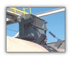
LONG WET OR DRY KILN SYSTEMS The mid-kiln valve is mounted on the kiln, at a location typically 50% to 60% the length of the kiln from the feed end. At this point, temperatures are high enough and residence times long enough to ensure complete combustion of the tire. Tire injection cycles are determined by kiln rotation. An AFS cam opens the valve smoothly, with minimum mechanical forces. The open dwell period is precise, and the closing is smooth and guiet, regardless of kiln diameter or speed.
